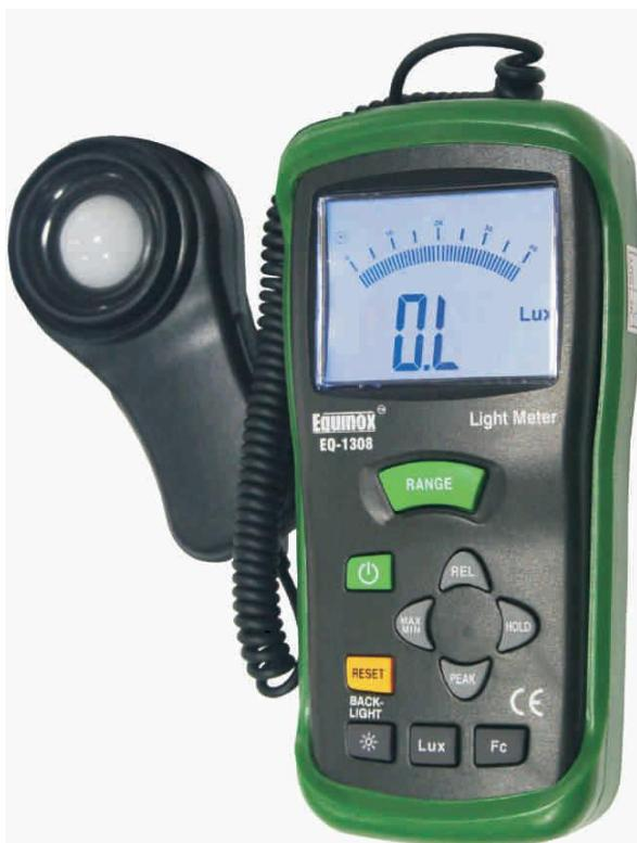
Instrument is easy to use with light weight, providing accurate display light level in terms of Foot Candles (FC) or LUX over wide range. Just turning the Function Switch to select the "Lux" scale and then Exposing the photo detector to light source in a horizontal position, thus the meter will display illuminance and LCD Display.
