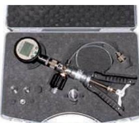
Die Digital test pressure gauges **LDM 70** are available as Complete Pressure Calibration kits (case, with Calibration Hand Pump LPP 30). The calibration Hand Pump LPP 30 Generates Pressure up to 500 psi (35 bar), switchable to Vacuum Generation -28 in Hg.
