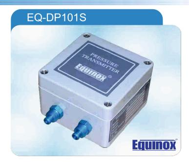
These are analog output transmitters, intended to use with non-corrosive, Gases or Air. The Piezo Resistive sensor gives extremely precise and stable measurements of the applied pressure, with excellent repeatability and better temperature stability. Various application to name are to monitor Clean Room pressure, Across filters, etc.
