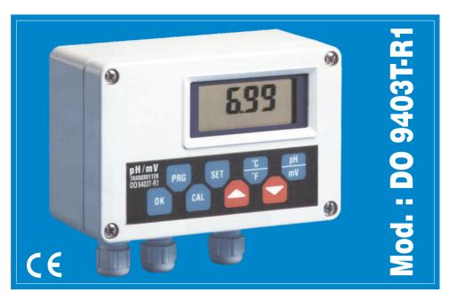
The DO 9403T-R1 pH transmitter converts the output of a pH electrode, with temperature compensation, into a signal at  $4\sim20$  mA. The pH or Redox electrode input circuit is galvanically insulated against the  $4\sim20$ mA output signal. An LCD indicator allows viewing of the process signal value and of the various parameters.
