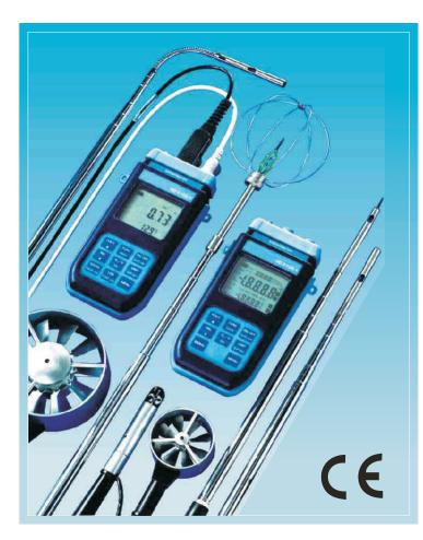
The HD2103.2 is a Portable Instrument with a large LCD display. It is designed for use in the fields of Air Conditioning, Heating, Ventilation & Environmental Comport. Hot-wire or Vane Probes are Used to Measure Air Speed, Flow Rate, & Temperature inside pipelines & vents.
